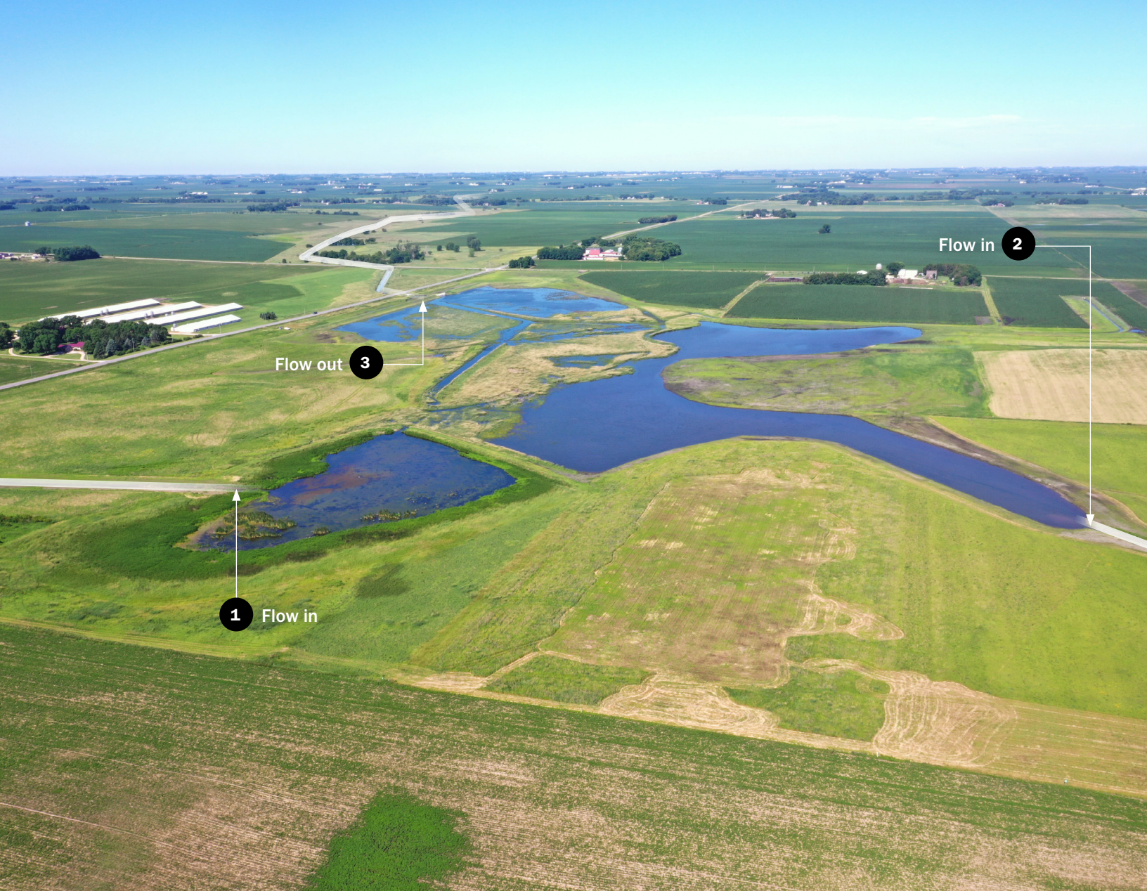
Figure 12: A shallow wetland storage basin that receives both surface and subsurface drainage.
